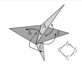
VF relation does not involve any dynamic allocation, the chain of face is distributed onto the involved face
